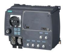
SIRIUS motor starter M200D technology module direct-on-line starter mechanical switching AC-3, 0.75 kW/400 V 0.15 A...2.00 A electronic overload protection thermistor: thermoclick / PTC without brake contact 4 DI / 2 DO Han Q4/2 - Han Q8/0 with manual on-site operation and keyswitch via communications module 3RK1305\* can be used on PROFIBUS or PROFINET
