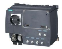
SIRIUS motor starter M200D technology module reversing starter mechanical switching AC-3, 0.75 kW/400 V 0.15 A...2.00 A electronic overload protection thermistor: thermoclick / PTC without brake contact 4 DI / 2 DO Han Q4/2 - Han Q8/0 via communications module 3RK1305\* can be used on PROFIBUS or PROFINET
