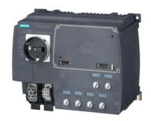
SIRIUS motor starter M200D technology module direct-on-line starter mechanical switching AC-3, 0.75 kW/400 V 0.15 A...2.00 A electronic overload protection thermistor: thermoclick / PTC without brake contact 4 DI / 2 DO Han Q4/2 - Han Q8/0 via communications module 3RK1305\* can be used on PROFIBUS or PROFINET
