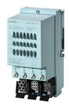
ET 200pro ERSE/RSSE HF electronic reversing starter electronic (soft-) switching Full motor protection consisting of: electronic Overload protection + thermistor AC-3, 5.5 kW / 400 V 1.5 A...(9 A)12 A Brake contact 400 V AC 4 DI Han Q4/2 - Han Q8/0
