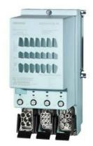
ET 200pro EDSE/DSSE HF electronic DOL starter electronic (soft-) switching Full motor protection consisting of: electronic Overload protection + thermistor AC-3, 5.5 kW / 400 V 1.5 A...(9 A)12 A Brake contact 400 V AC 4 DI Han Q4/2 - Han Q8/0
