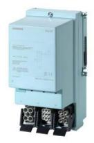
ET 200pro RSE ST Reversing starter standard Mechanical switching Electronic overload protection AC-3, 5.5 kW / 400 V 1.50 A...12.00 A without brake contact Han Q4/2 - Han Q8/0
