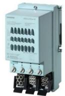
ET 200pro ERSE/RSSE HF electronic reversing starter electronic (soft-) switching Full motor protection consisting of: electronic overload protection + thermistor 400 V 3 AC/0.9 kW 0.15 A...2.00 A Brake contact 400 V AC 4 DI Han Q4/2 - Han Q8/0
