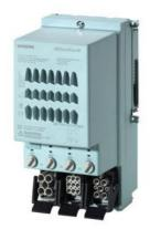
ET 200pro ERSE/RSSE HF electronic reversing starter electronic (soft-) switching Full motor protection consisting of: electronic overload protection + thermistor 400 V 3 AC/0.9 kW 0.15 A...2.00 A without brake contact 4 DI Han Q4/2 - Han Q8/0
