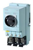
ET 200pro F-RSM Safety local Maintenance switch module Up to 16 A Disconnector function for Main circuit and safety evaluation functions Han Q4/2
