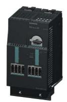
RS1E-X for ET200S High Feature reversing starter Setting range 2.4...8 A Mechanical switching Electronic protection AC-3, up to 3 kW / 400 V expandable for Brake control module 2DI module 2DI module Motor starter ES Circuit breaker signaling parameterizable DPV 1-capable PROFIENERGY-capable to PN
