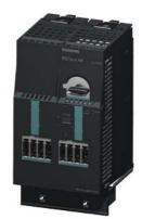
F-RS1E-X for ET 200S Failsafe reversing starter Setting range 0.3...3 A Mechanical switching Electronic protection expandable for Brake control module 2DI module 2DI module Circuit breaker signaling parameterizable
