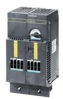
F-RS1E-X for ET 200S Failsafe reversing starter Setting range 0.3...3 A Mechanical switching Electronic protection AC-3, up to 1.1 kW / 400 V expandable for brake control module for 2DI control module
