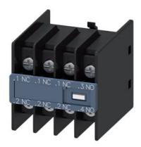
auxiliary switch, on the front, 1 NO + 3 NC, .1/.2, .1/.2, .1/.2, .3/.4, current path: 1 NC, 1 NC, 1 NC, 1 NO, ring cable lug connection, for contactors 3RT2 and contactor relays 3RH2
