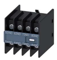
auxiliary switch, on the front, 4 NO, 53/54, 63/64, 73/74, 83/84, current path: 1 NO, 1 NO, 1 NO, 1 NO, ring cable lug connection, physically coded, only with contactor relays 3RH2140 and 3RH2444 combinable (according to EN 50011)
