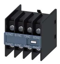
auxiliary switch, on the front, 3 NO + 1 NC, 53/54, 61/62, 73/74, 83/84, current path: 1 NO, 1 NC, 1 NO, 1 NO, ring cable lug connection, physically coded, only with contactor relays 3RH2140 and 3RH2443 combinable (according to EN 50011)
