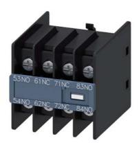
auxiliary switch, on the front, 2 NO + 2 NC, 53/54, 61/62, 71/72, 83/84, current path: 1 NO, 1 NC, 1 NO, ring cable lug connection, physically coded, only with contactor relays 3RH2140 and 3RH2442 combinable (according to EN 50011)
