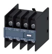
auxiliary switch, on the front, 4 NO, .3/.4, .3/.4, .3/.4, .3/.4, current path: 1 NO, 1 NO, 1 NO, 1 NO, ring cable lug connection, for contactors 3RT2 and contactor relays 3RH2
