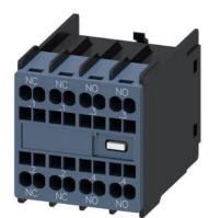
auxiliary switch, on the front, 2 NO + 2 NC, .1/.2, .1/.2, .3/.4, .3/.4, current path: 1 NC, 1 NC, 1 NO, 1 NO, spring-loaded terminal, for contactors 3RT2 and contactor relays 3RH2
