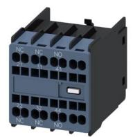
auxiliary switch, on the front, 1 NO + 2 NC, 21/22, 31/32, 43/44, --/--, current path: 1 NC, 1 NC, 1 NO, --, spring-loaded terminal, for contactors 3RT2 and contactor relays 3RH2
