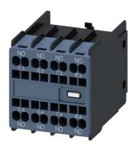
auxiliary switch, on the front, 4 NO, 53/54, 63/64, 73/74, 83/84, current path: 1 NO, 1 NO, 1 NO, 5 N
