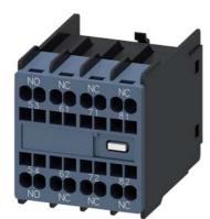
auxiliary switch, on the front, 1 NO + 3 NC, 53/54, 61/62, 71/72, 81/82, current path: 1 NO, 1 NC, 1 NC, 1 NC, spring-loaded terminal, physically coded, only with contactor relays 3RH2140 and 3RH2440 combinable (according to EN 50011)
