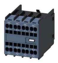
auxiliary switch, on the front, 4 NC, 51/52, 61/62, 71/72, 81/82, current path: 1 NC, 1 NC, 1 NC, 1 NC, spring-loaded terminal, physically coded, only with contactor relays 3RH2140 and 3RH2440 combinable (according to EN 50011)
