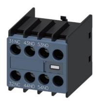
auxiliary switch, on the front, 2 NO + 1 NC, 31/32, 43/44, 53/54, --/--, current path 1 NC, 1 NO, 1 NO, --, screw terminal, for contactors 3RT2 and contactor relays 3RH2
