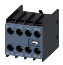
auxiliary switch, on the front, 4 NO, 53/54, 63/64, 73/74, 83/84, current path: 1 NO, 1 NO, 1 NO, 1 NO, screw terminal, for contactors 3RT2 and contactor relays 3RH2
