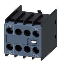
auxiliary switch, solid-state compatible, on the front, 2 NC, .1/.2, --/--, .-/-, .1/.2, current path: 1 NC (solid-state compatible), --, --, 1 NC (solid-state compatible), screw terminal, for contactors 3RT2 and contactor relays 3RH2
