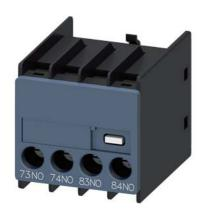
auxiliary switch, on the front, 2 NO, 73/74, 83/84, current path: 1 NO, 1 NO, cable entry from below, screw terminal, for contactors 3RT2 and contactor relays 3RH2
