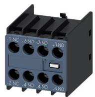
auxiliary switch, on the front, 3 NO + 1 NC, .1/.2, .3/.4, .3/.4, .3/.4, current path: 1 NC, 1 NO, 1 NO, 1 NO screw terminal, for contactors 3RT2 and contactor relays 3RH2
