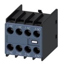
auxiliary switch, on the front, 1 NO + 3 NC, .1/.2, .1/.2, .3/.4, current path: 1 NC, 1 NC, 1 NC, 1 NO, screw terminal, for contactors 3RT2 and contactor relays 3RH2
