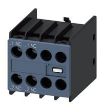
auxiliary switch, on the front, 2 NC, .1/.2, .1/.2, .-/--, current path: 1 NC, 1 NC, --, --, screw terminal, for contactors 3RT2 and contactor relays 3RH2
