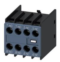
auxiliary switch, on the front, 2 NO + 2 NC, 22 U, .7/.8, .7/.8, .5/.6, .5/.6, current path: 1 NO (leading), 1 NO (leading), 1 NC (lagging), 1 NC (lagging), screw terminal, for contactors 3RT2 and contactor relays 3RH2
