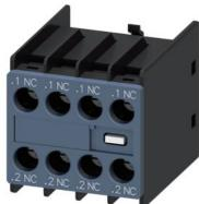
auxiliary switch, on the front, 4 NC, .1/.2, .1/.2, .1/.2, .1/.2, current path: 1 NC, 1 NC, 1 NC, 1 NC, 1 NC, screw terminal, for contactors 3RT2 and contactor relays 3RH2
