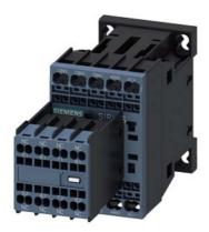
Contactor relay, 4 NO + 4 NC, 24 V DC, Size S00, spring-type terminal, Removable auxiliary switch
