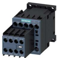
Contactor relay, 4 NO + 4 NC, 110 V AC, 50 / 60 Hz, Size S00, screw terminal, Removable auxiliary switch
