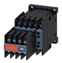
contactor relay, 4 NO + 4 NC, 110 V AC, 50 Hz / 120 V, 60 Hz, size S00, ring cable lug connection, captive auxiliary switch
