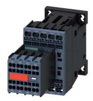
contactor relay, 4 NO + 4 NC, 230 V AC, 50 / 60 Hz, size S00, spring-loaded terminal, captive auxiliary switch
