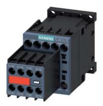
contactor relay, 4 NO + 4 NC, 230 V AC, 50 / 60 Hz, size S00, screw terminal, captive auxiliary switch
