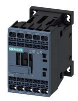
Contactor relay for railway 4 NO DC 72-125V, 0.7...1.25\*US, with integrated varistor Size S00, Spring-type terminal suitable for PLC outputs
