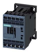
Contactor relay, 4 NO, 24 V DC, with integrated diode, Size S00, Spring-type terminal
