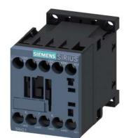
Coupling contactor relay, 4 NO, 24 V DC, 0.7  $\dots$  1.25\* US, Size S00, screw terminal suitable for PLC outputs
