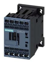
Contactor relay, 3 NO + 1 NC, 110 V AC, 50 / 60 Hz, with full-wave rectifier, Size S00, Spring-type terminal
