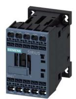
Coupling contactor relay, 2 NO + 2 NC, 24 V DC, 0.85  $\ldots$  1.85\* US, with integrated diode, Size S00, Spring-type terminal
