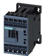
Coupling contactor relay, 2 NO + 2 NC, 110 V DC, 0.7 ... 1.25\* US, with integrated suppressor diode, Size S00, Spring-type terminal suitable for PLC outputs
