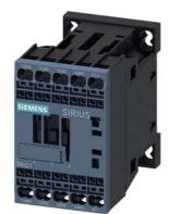
Coupling contactor relay, 2 NO + 2 NC, 24 V DC, 0.7 ... 1.25\* US, with integrated suppressor diode, Size S00, Spring-type terminal suitable for PLC outputs
