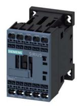
Coupling contactor relay, 2 NO + 2 NC, 24 V DC, 0.7 ... 1.25\* US, Size S00, Spring-type terminal suitable for PLC outputs
