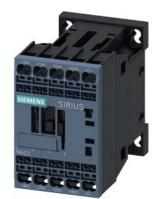
Contactor relay, 2 NO + 2 NC, 24 V DC, with integrated diode, Size S00, Spring-type terminal
