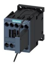
Contactor relay railway, 2 NO + 1 NC 220 V DC, 0.7 ...  $1.25^*$  US, with integrated suppressor diode, Size S00, screw terminal installation on standard mounting rail optimized (20 G) suitable for PLC outputs
