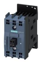
Solid-state contactor 3-phase 3RF3 AC 53 / 5.2 A / 40  $^{\circ}\text{C}$  48-480 V / 110-230 V AC 2-phase controlled Instantaneous switching Spring-type terminal
