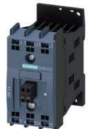
Solid-state contactor 3-phase 3RF3 AC 53 / 5.2 A / 40  $^\circ C$  48-600 V / 24 V DC 2-phase controlled Instantaneous switching Spring-type terminal
