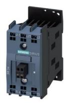
Solid-state contactor 3-phase 3RF3 AC 53 / 5.2 A / 40  $^{\circ}\text{C}$  48-480 V / 24 V DC 2-phase controlled Instantaneous switching Spring-type terminal
