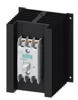
Solid-state contactor 3-phase 3RF2 AC 51 / 50 A / 40  $^{\circ}$ C 48-600 V / 4-30 V DC 3-phase controlled Ring cable connection Blocking voltage 1200 V
